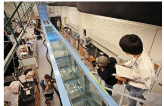
The 36-meter wave tank in Chapman Hall allows researchers and students to study fluid dynamics, turbulence and other phenomena.
